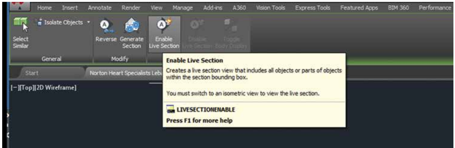
Figure 5: Live Section view
