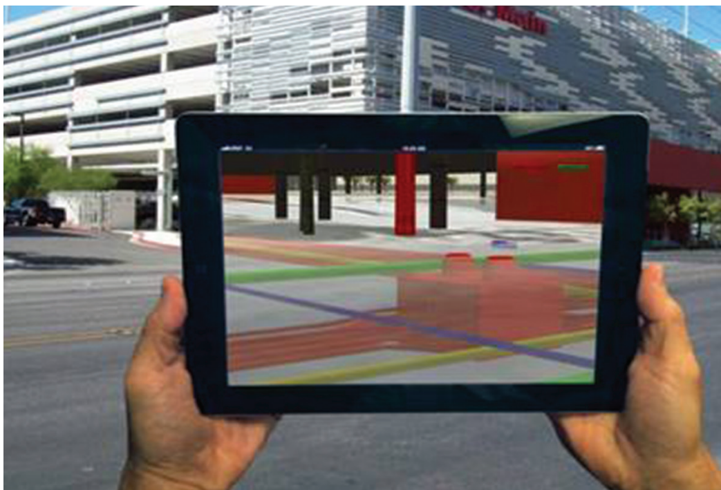
Figure 7: The use of Reality Computing to support augmented reality will enable municipal and utility workers to visualize underground utilities superimposed over real images of a street. Image courtesy of VTN.
