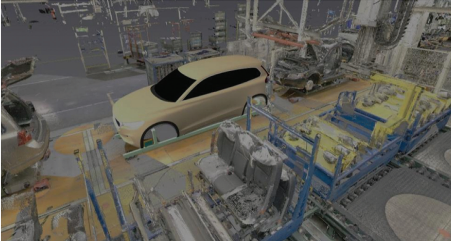
Figure 6: Automotive manufacturers use reality scanned data to capture existing conditions of factories and assembly lines. Image courtesy of Volvo Car Group.
