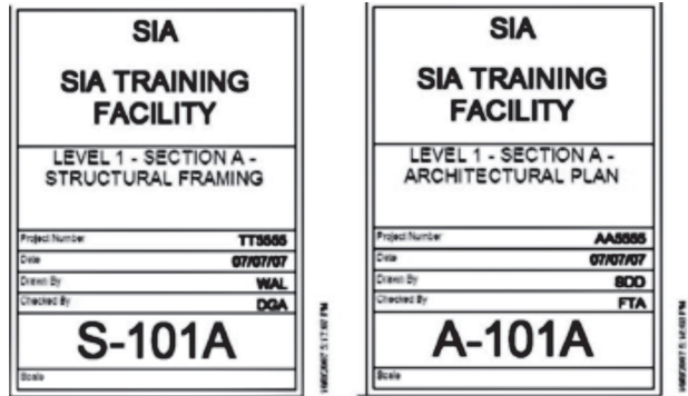
Figure 1: Examples of structural and architectural coordinated sheets.
