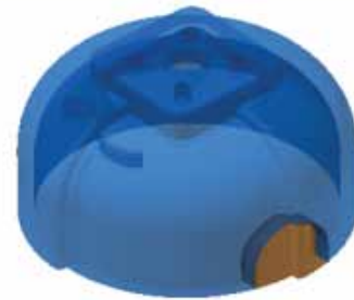
Figure 34: Included surfaces in derived plastic part
