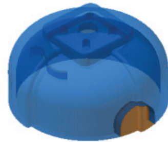
Figure 34: Included surfaces in derived plastic part
