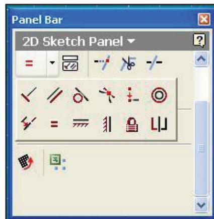
Figure 1: Constraint Toolbar
