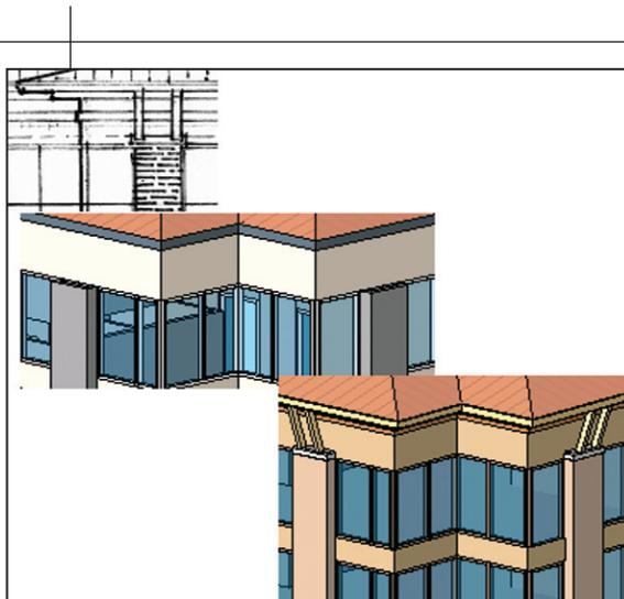
Figure 2 – Development of the roof, soffit, eaves, and column caps from sketch to generic wall-to-wall combined with in-place family in a group.
