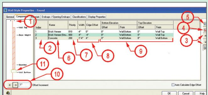
Figure 7 Component Tab of Wall Style Properties
